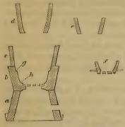
and powerful. The furnace is made out of fragments of broken blue pots, and consists of several parts, sections of which are here given, drawn upon a scale of one inch to ten. The lower piece a is fitted into a tin bottom, consisting of a circular plate with a rising rim; the junction being made tight by plaster of Paris. The piece b, rest-
